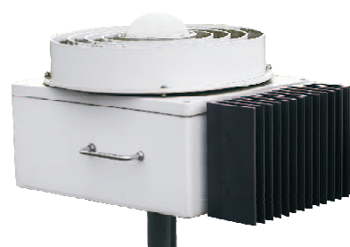
Temperature stabilized choke ring antenna
